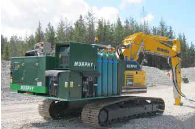
Figure 7. Weld equipment mounted on backhoe.
